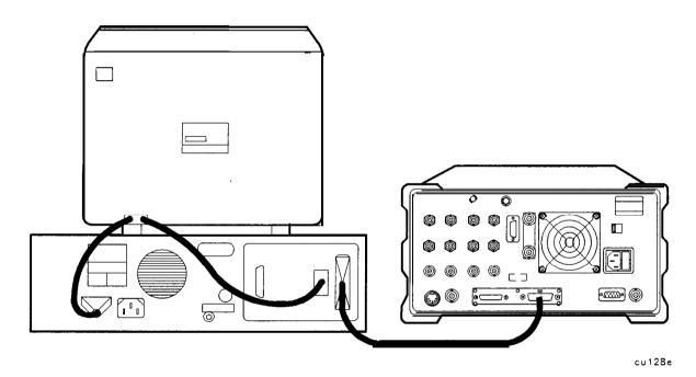
Figure 1-1. Connecting the HP 9000 Series 200 Computer to the Spectrum Analyzer
