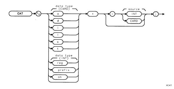
Equivalent Softkeys: the functions accessed by Catalog Internal or Catalog Card. Related Commands: LOAD, MSI, STOR.
