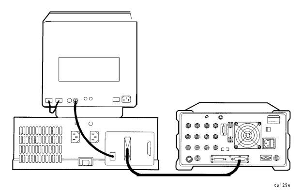
Figure 1-4. Connecting the Personal Computer to the Spectrum Analyzer
